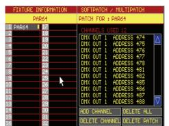
When a dimmer or spot is taken, and instead of selecting an address, the *MULTIPATCH function is activated*, a softpatch window will open.
